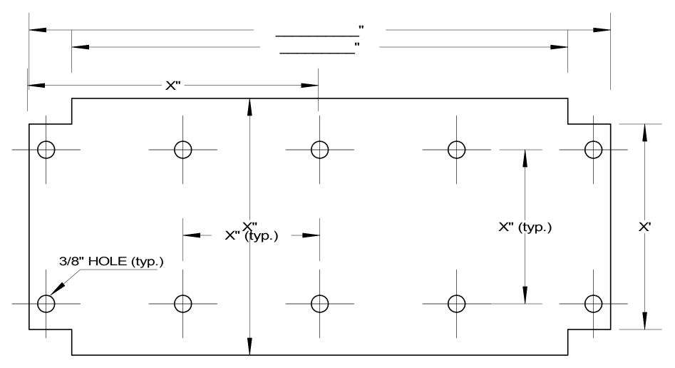
MADE FROM 3/16" THICK PLATE SLUG TEMPLATE 2
